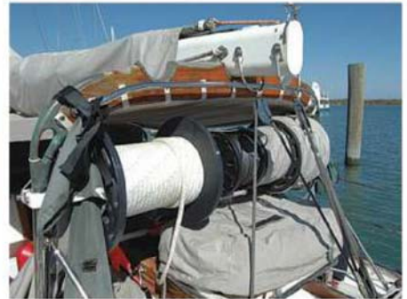
Hard around but secured in place by the anchor rode and lines run to the pier, Beatrix and her crew wait anxiously for the tide to turn (left); Reels with plenty of line on them are permanently mounted aft of the cockpit (right)
